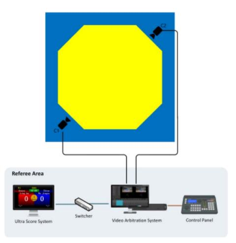
4 channels synchronize video record. Track back or slowmotion playback each channel even during the recording.
