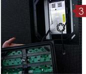
Signal transmission to each individual module is separate, improving screen's visual perfor-mance and simplifying the trouleshooting process.
