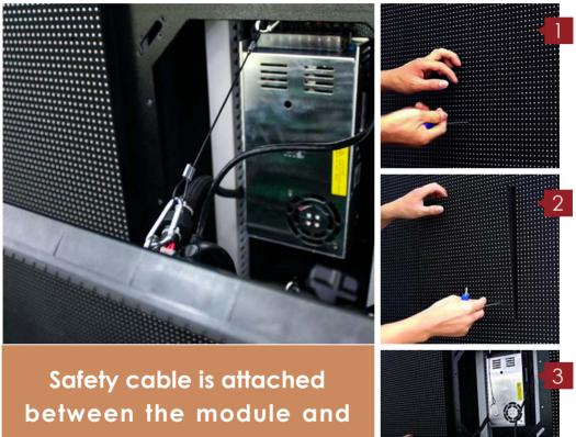
cabinet to prevent damage from falling during service.
