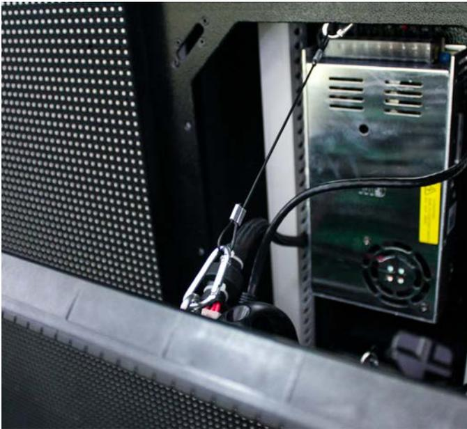
**Safety cable is attached between the module and cabinet to prevent damage from falling during service.**
