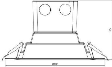
**Size :  $\Phi 195 \times 115 \text{mm} (7.72 \times 4.53 \text{''})$**
